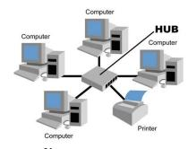
Star Network - Each PC is connected to the server by a cable.
