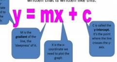
So the graph of y = 2x + 5 will cross the y axis at + 5 and will have a gradient of 2. Key Point - If two lines are <u>parallel</u> they will have the <u>same gradient</u>.
