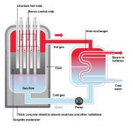
The main nuclear fuels are **uranium** and **plutonium**. In a nuclear power station nuclear fuel undergoes a controlled chain reaction in the reactor to produce heat - nuclear to heat energy.
