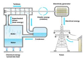
In a thermal power station fuel such as coal, oil or gas is burned in a furnace to produce heat - chemical to heat energy.
