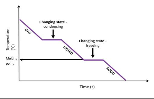
As a pure substance changes state, the temperature remains constant, this is called the melting or boiling point.
