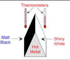
Shiny white surfaces are the best at reflecting infrared radiation
